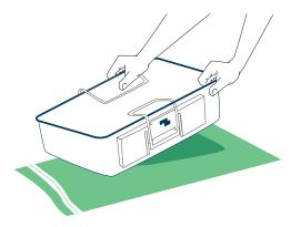
**Step 3:** Place the lid on the rigid sterilization container and close the latches.
