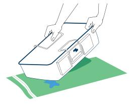
**Step 5:** If the container leaks, note that this is leakage through the gasket seal, which indicates a defect in the seal or in the latching mechanism.
